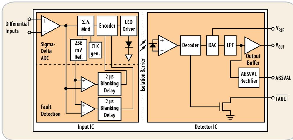
**Figure 2:** In the HCPL-788J iso-amp, the differential input voltage is digitally encoded by a sigma-delta A/D converter and then fed to the LED driver, which sends the data across the isolation barrier to a detector and D/A.
